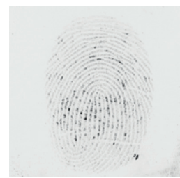
c) Example of a too-dry finger
