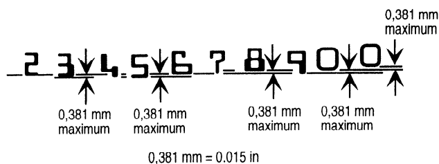
Figure 17 — Allowable variation in vertical alignment
