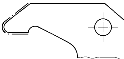
Figure 38 — Indication of a combination of adjoining features
