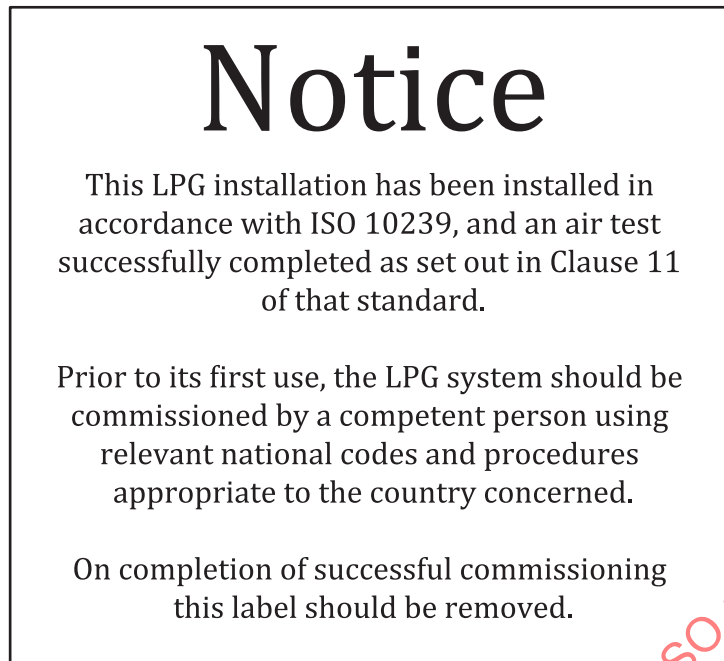
Figure 2 — Specifications for an LPG system commissioning label
