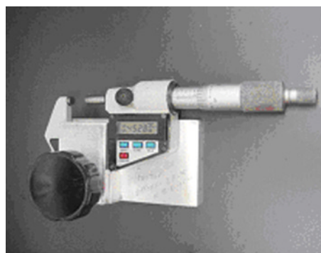
Figure 8 — Micrometer mounted to adapter
