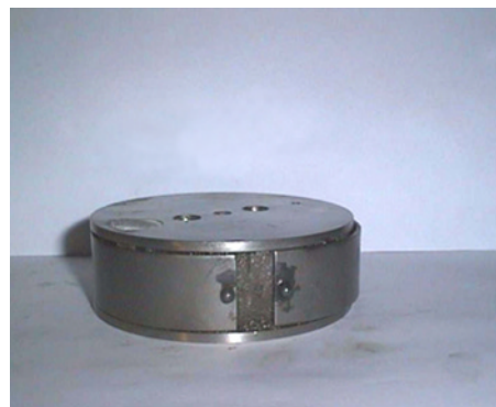
Figure 2 — Typical mould assembly (side view)
