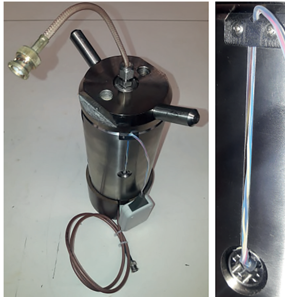
Figure A.2 — Modified UCA vessel with on the right a zoom-in on the slot for transducer cables (outside view)
