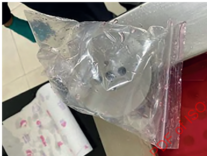
Figure 11 — Ring mould inserted in a re-sealable bag
