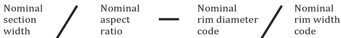
Figure 1 — — Indication of dimensional and constructional characteristics
