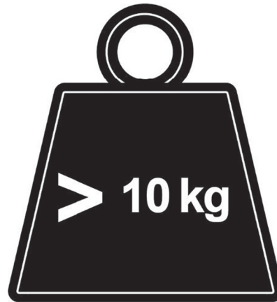
Figure 8 — Example of graphical symbol for parts weighing more than 10 kg (application of ISO 7000-1321B)
