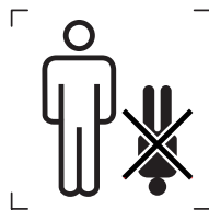
Figure 5 — Example of marking of stretcher head end and foot end (ISO 7000-3851)
