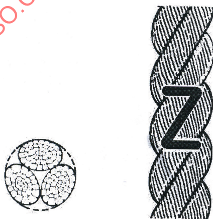
Figure 1 — Shape of a 3-strand hawser-laid rope (type A)
