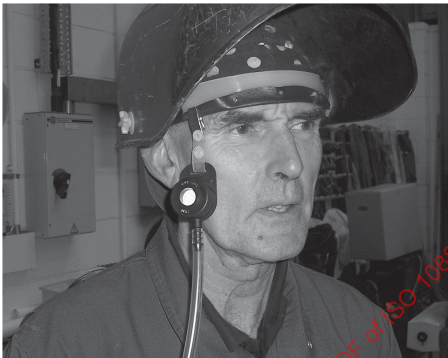
Figure B.4 — Sampler attached to the headband by means of its collar clip
