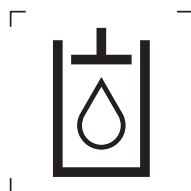
Figure 10 — Hydraulic filling point
