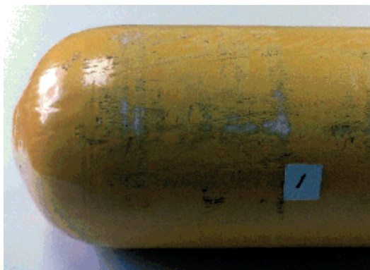
a) Level 1 abrasion damage — Superficial abrasion
