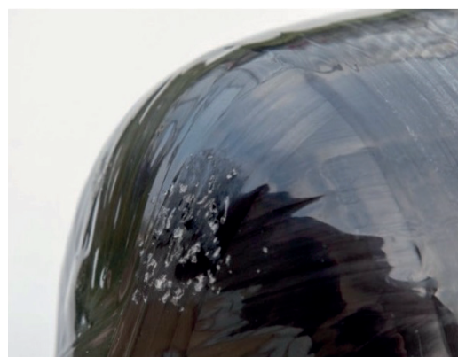
a) Examples of Level 1 impact damage — Superficial impact damage
