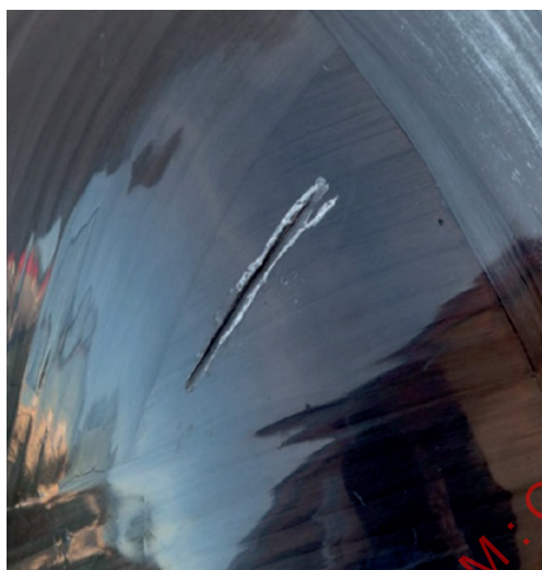
c) Examples of Level 3 damage from cuts and showing device for cut depth measurement
