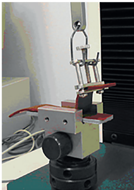
Figure 5 — Arrangement of test specimen and clamps for test with flat-jawed clamp system
