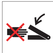
Figure D.27 — Do not reach into crushing area
