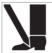
Figure C.13 — Cutting of foot
