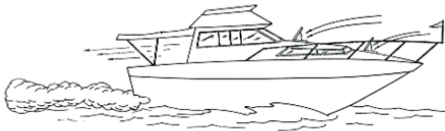
a) Desired airflow through the boat
