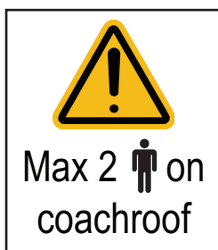
Figure B.2 — Limited access (using ISO 7010 – W001 “General warning”)
