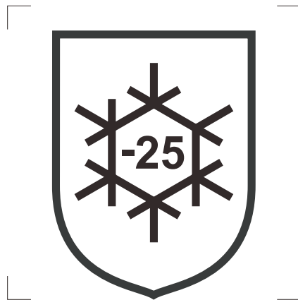
Figure 1 — Example of graphical symbol for cold environment for -25°C [IEC 60417-6292]
