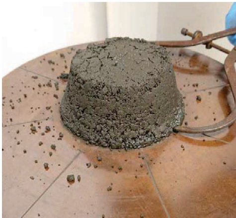
Figure 2 — Example of the material at the flow point (left) and at the flow point showing a moisture trail on the flow table (right)
