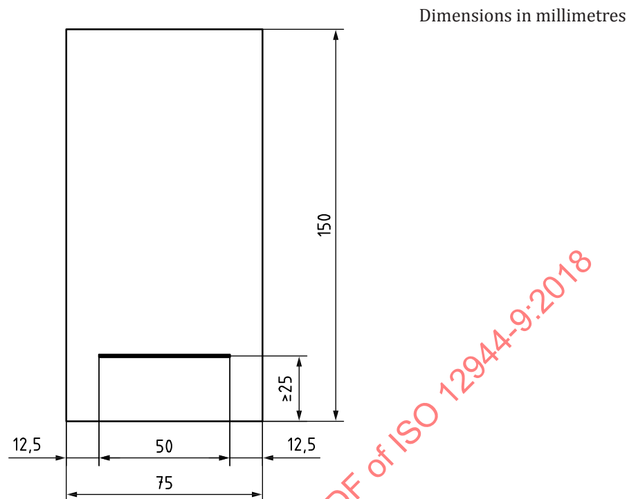
Figure A.2 — Example of test panel showing position of scribe line
