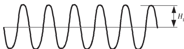
Figure 106 — Interference signal at 16 Hz and 50 Hz
