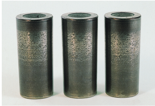
Figure 31 — Indentations from particles on tapered rollers
