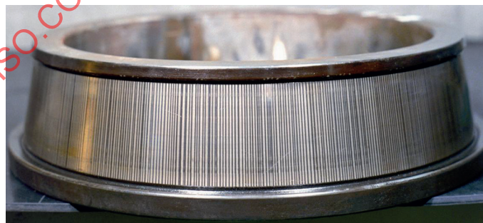
Figure 23 — Fluting (washboarding) as a result of current leakage on the inner ring raceway of a tapered roller bearing
