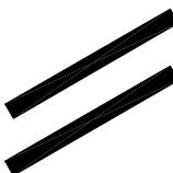
Figure 2 — Symbol for inclined joint
