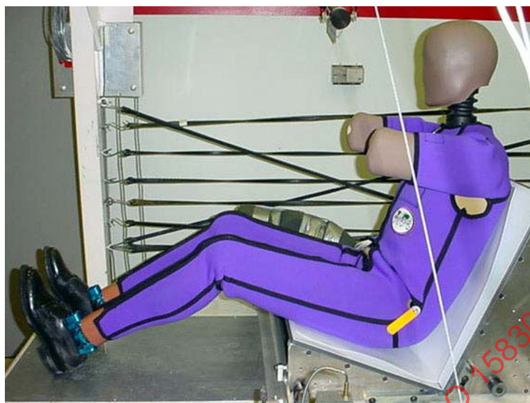
Figure 7 — Side view of setup for full dummy certification tests
