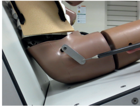
Figure 25 — Reference hole on H-point tool
