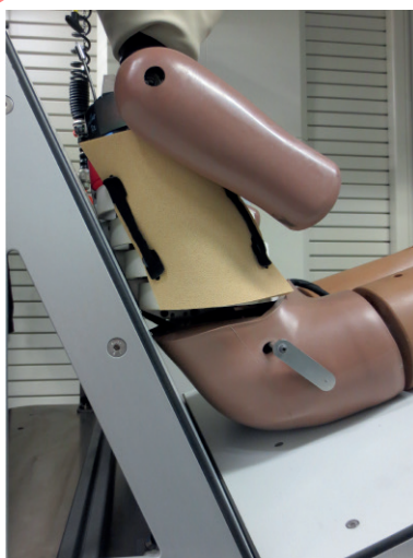
Figure 20 — H-point tool installed on the right side
