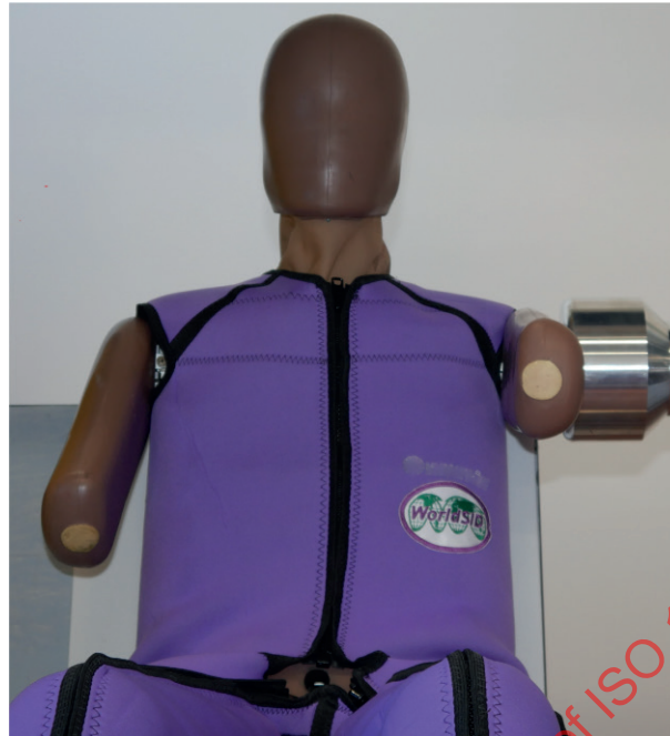
Figure 14 — Shoulder test, dummy and arm position
