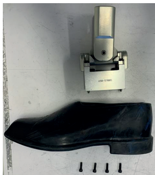
Figure A.68 — Moulded shoe removed from ankle assembly
