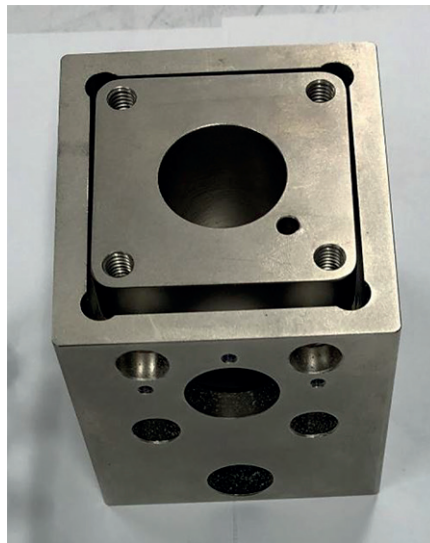
Figure A.45 — Lumbar spine load cell structural replacement placed into sacroiliac structural replacement
