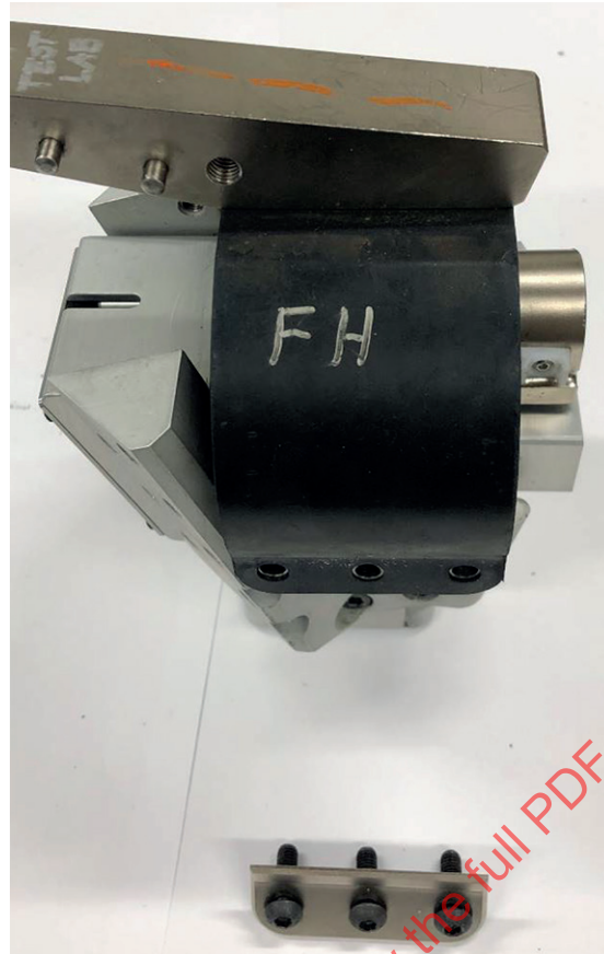
Figure A.48 — Attach lumbar lower clamping plates
