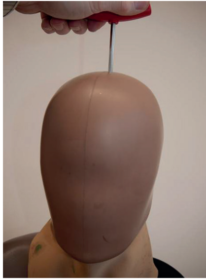
Figure A.3 — Removal of moulded head
