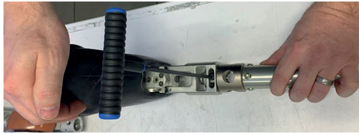
Figure A.66 — Removal of z-axis radial limit screw
