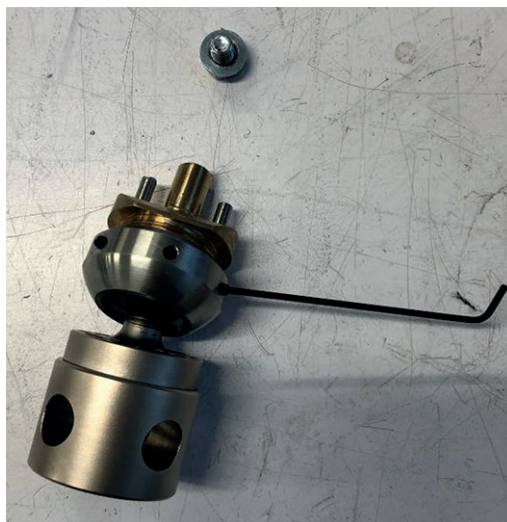
Figure A.57 — Remove hip joint socket
