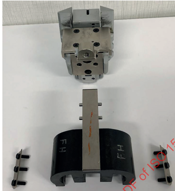
Figure A.40 — Lumbar spine assembly removed from sacroiliac assembly
