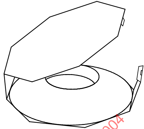
Figure C.6 — Card cover with integral plastic pitfall and absorbent pad for attractant oil
