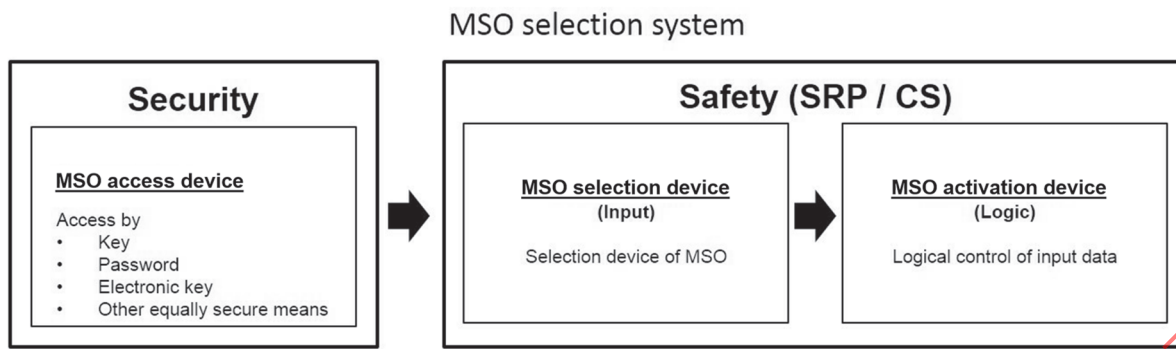
Figure 1 — Border between security system and safety system
