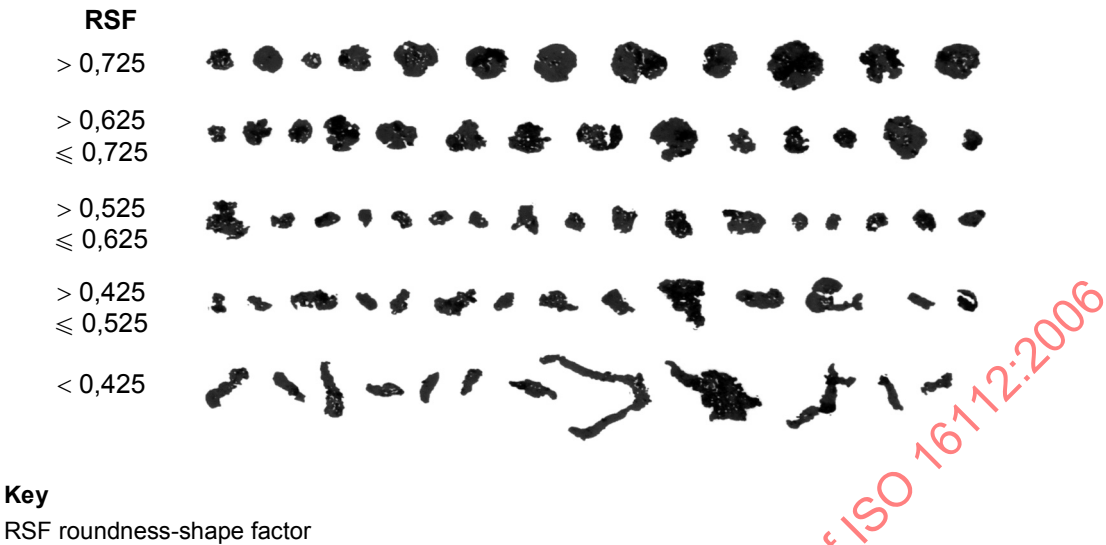
Figure B.3 — Visual representation of graphite particles categorized by roundness-shape factor
