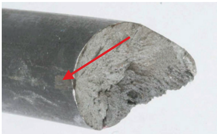
Figure C.4 — Mechanical damage on the rod surface (indicated by the arrow)
