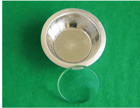
Figure 7 — Fused bead after completion of fusion process
