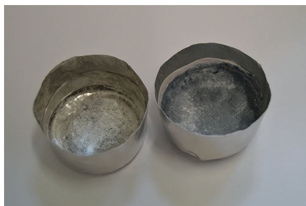
Figure 2 — Appearance of mixture prior to sintering (left) and after successful sintering (right)
