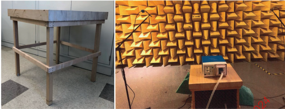
a) Example standard test table based on ISO 7779:2018, Annex A
