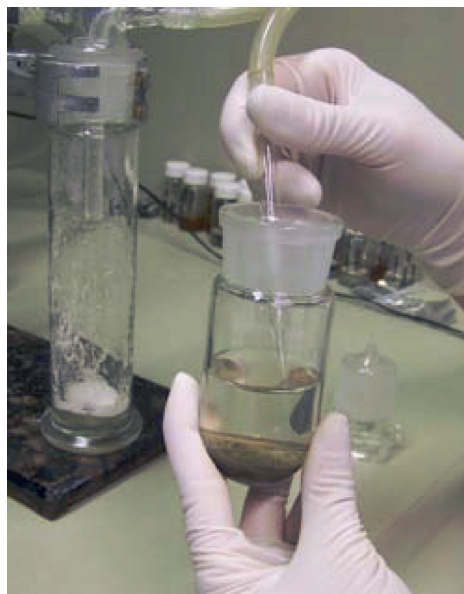
Figure B.5 — Tenax® beads are collected using a Pasteur pipet and suction
