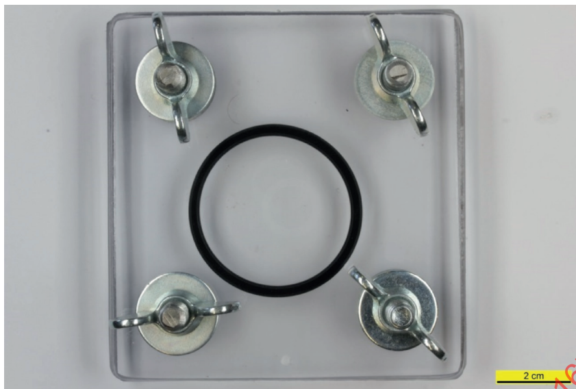
Figure C.2 — compression of O-ring using 4 screws
