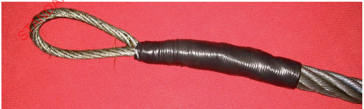
Figure 2 — Completed flexible pulling eye made from the steel core itself
