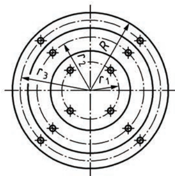
Figure 2 — Air velocity measuring points of round duct
