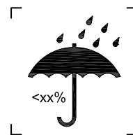
Figure 4 — Maximum humidity of storage conditions
