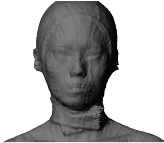
Figure 4 — An inappropriate scan result with significant noise
