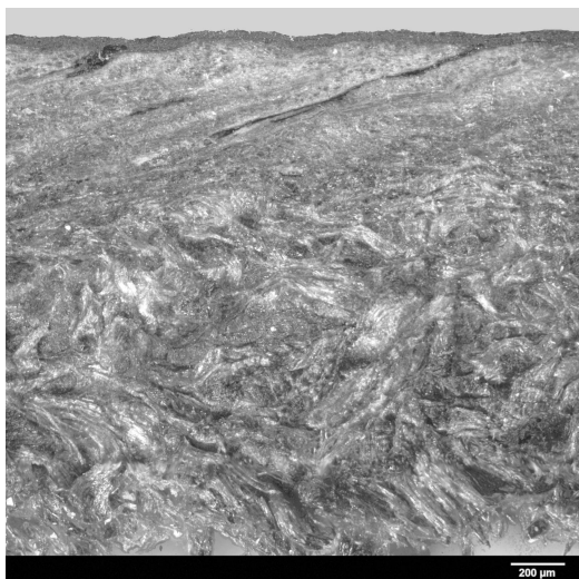
Figure B.1 — Typical section of bovine leather with surface coating of less than 150 µm
