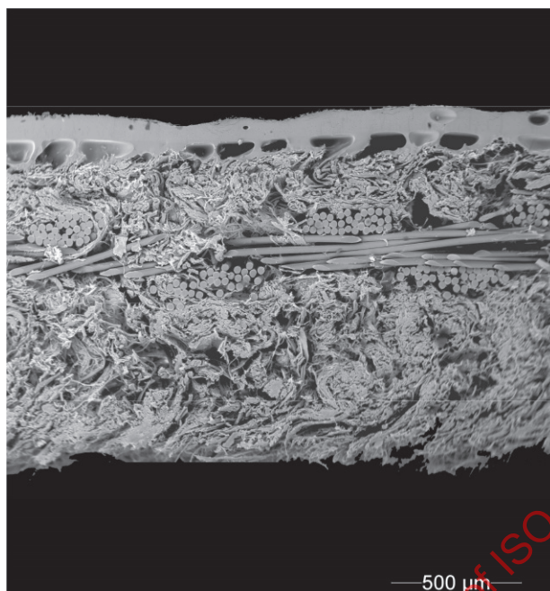
Figure A.11 — Section of textile material coated with leather fibres
