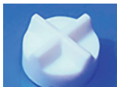
Figure 1 — Cowie double crosshead stir bar (typical dimensions: 20\text{ mm} < d < 25\text{ mm} , 12\text{ mm} < h < 18\text{ mm} )
