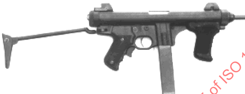
Figure A.14 — Submachine gun with blow-back action
