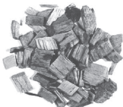
a) Wood chips (cut with sharp tools)
