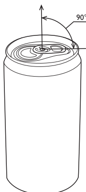
Figure B.7 — Illustration of mechanical tensile measurement
