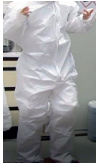
The garment is too loose. Additionally, the hands and feet are covered by garment and the crotch is closer to the knees because the height of the test subject is less than 150 cm.
