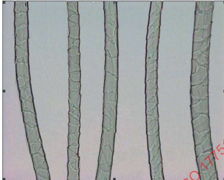
Figure C.28 — Irregular annular scales with large warping angles
