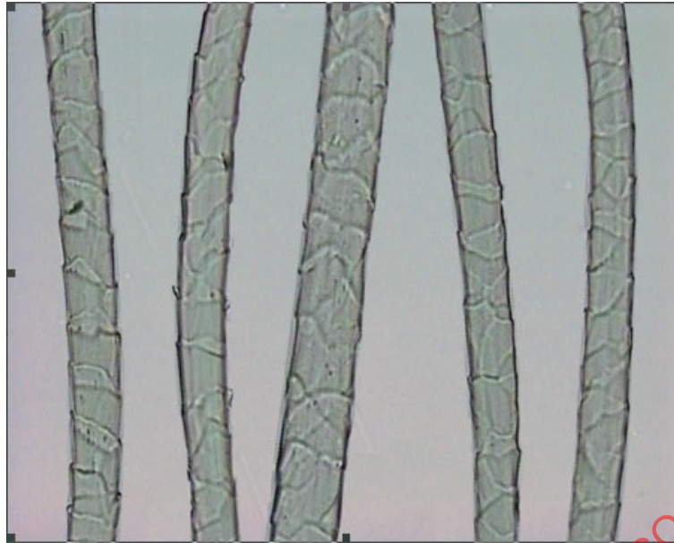
Figure C.30 — Irregular annular scales with thicker scale edges and high scale frequency
