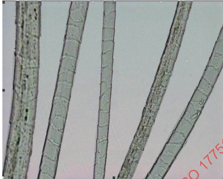
Figure C.16 — Regular ring-shaped scales with thin and smooth edges, scale frequency is low
