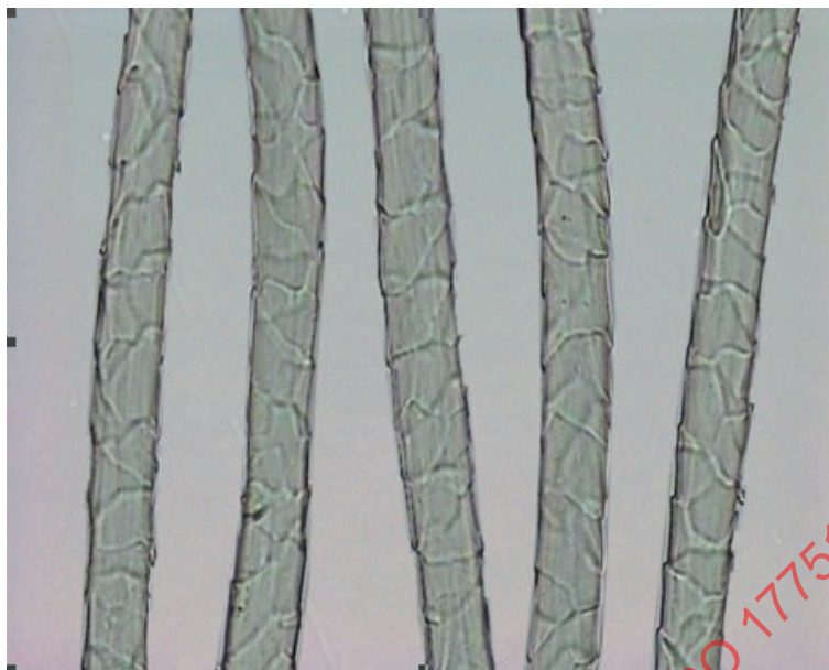
Figure C.32 — Scales are thick and fibre surfaces are rough
