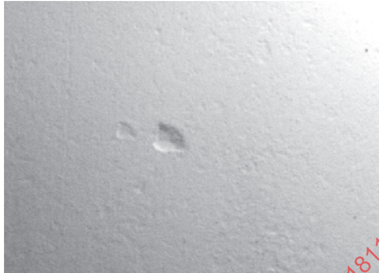
Figure B.5 — Isolated pits
