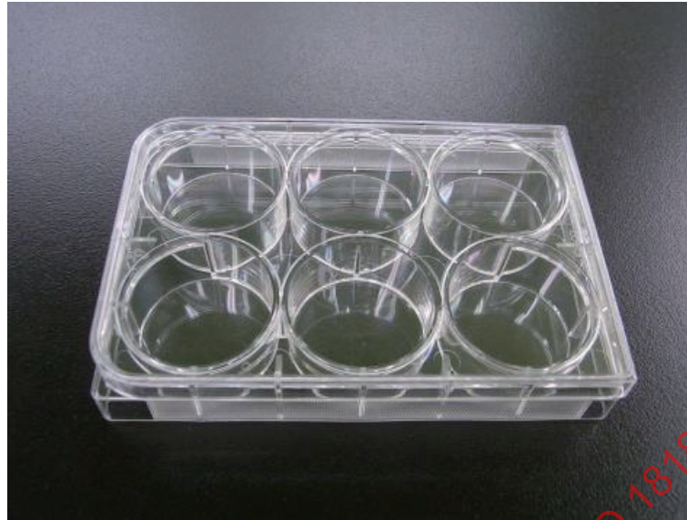
Figure 2 — 6 wells plastic plate for plaque assay
