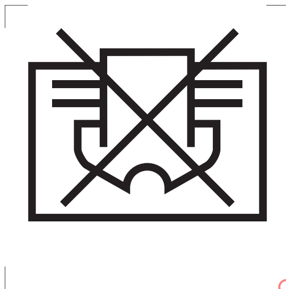
Figure G.3 — Not suitable for covering
