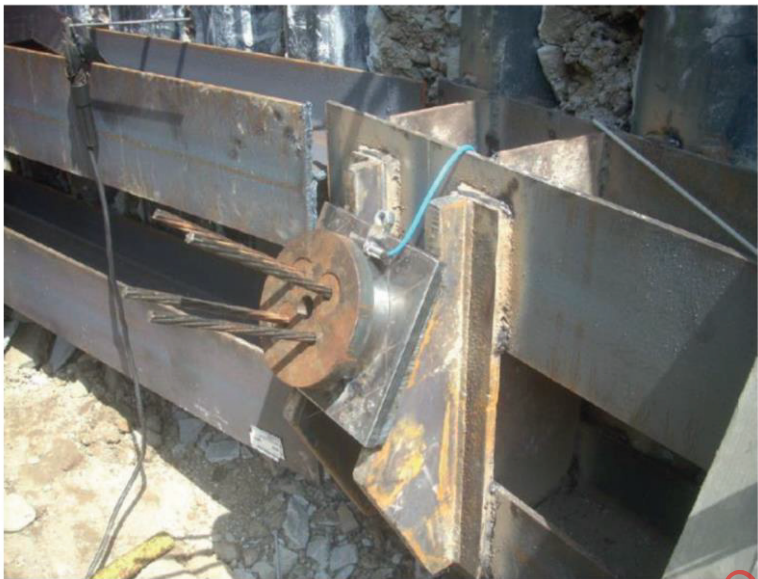
Figure B.2 — Electric load cell on steel beam with load distribution plates for an anchor with multiple strand tendons
